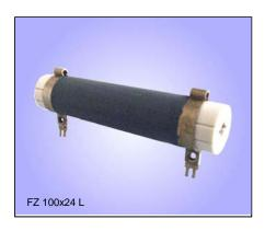
Cemented wirewound tubular fixed resistor, degree of protection IP00, for soldering on printed circuit boards, mounting and connection by soldering clips horizontal to mounting surface. Connections pretinned.
