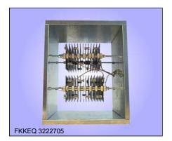
Steel-grid fixed resistor unit, degree of protection IP 00 integrated in a duct section for integration by the user into existing or new exhaust air installations, in a zinc steel sheet duct with attached terminal box and optional temperature switch.
