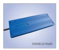
Short-circuit proof wirewound flat resistor with degree of protection IP 54 in blue anodized aluminium enclosure. Design with screened cable 3x1,3 mm² (AWG 16/19), 200°C, 0,75 m long.
