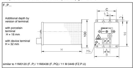
Example: Continuous dissipation 3x150W, resistance value  $3x120\Omega$ , star point in the device (connection at 3 porcelain terminals)
